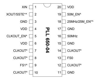
Note: ^: Internal pull-up resistor \*: Bi-directional pin °: Low EMI output
